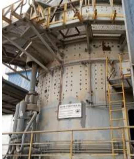
**Gambar 4.4** *Vertical Roller Mill*
