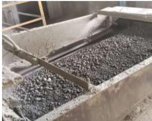
**Gambar 4.3** *Weight Feeder Clinker*
