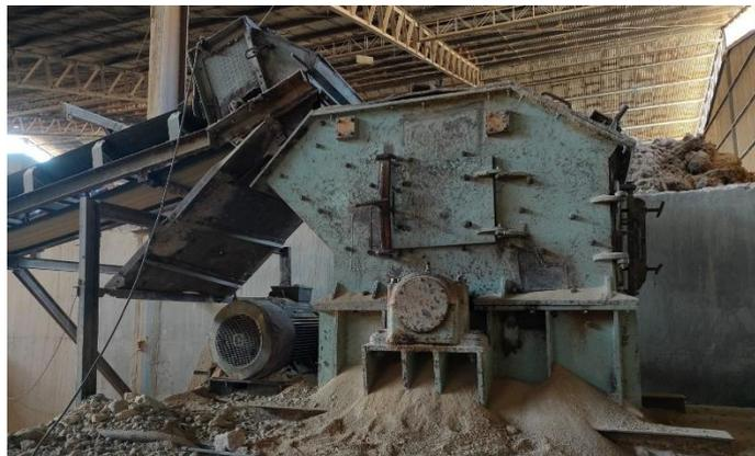
**Gambar 3.4** *Pig Crusher*
