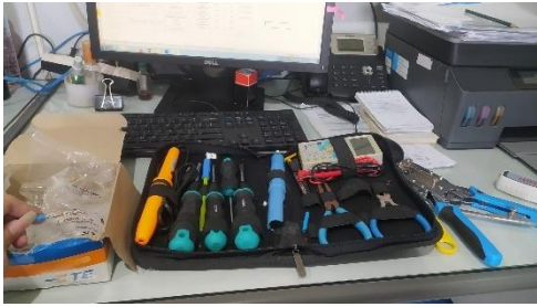
Gambar 1. Toolkit crimping kabel LAN RJ45
