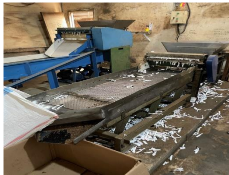
Gambar 4.5 Proses Mesin Reject Separator
